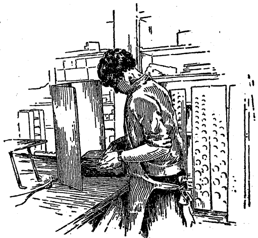
Testing leathers used in Electric-Pneumatic Action. Electric light reveals the slightest flaw.
