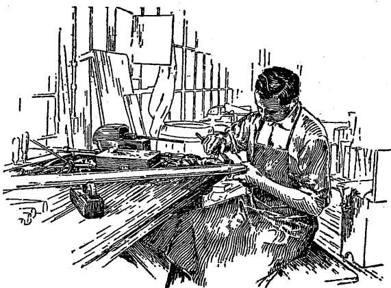
Soldering pipe foot to pipe body on metal pipe.
